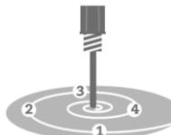
Dip the stick into 4 different zones before placing it back into the tube.
